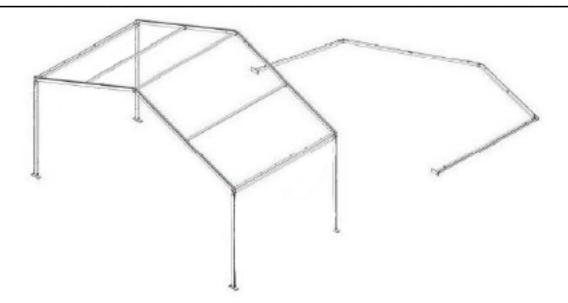
• Erect all frames and put the purlins on the roof as the first section. Place the portal beams like shown below opposite each other and on different sections.
