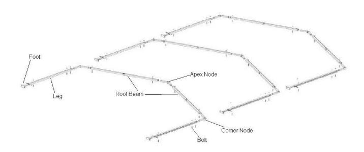
• Use the bolt to connect the Foot-Plates, Upright-Supports, Roof-Beams, Eave-Connections and Top Connections. And then, erect the first frame of the tent.
