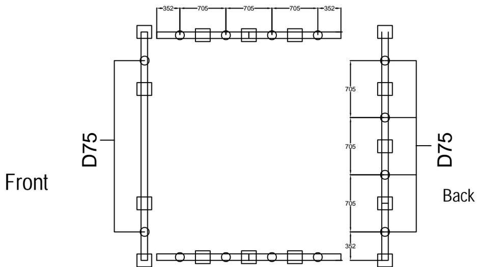
First lay out the cills, connectors and anchor brackets approximately in place, then tighten them with bolts and nuts which provided.
