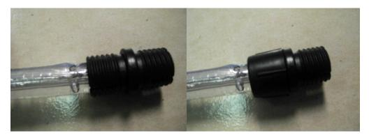
STEP 3 (NOTICE: When two sections are connected, try to switch it on and check whether the rope light works or not, if the rope lights does not work, simply remove the connector from rope light and turn the rope light or connector 180 degree as to correctly match the positive and negative poles).
